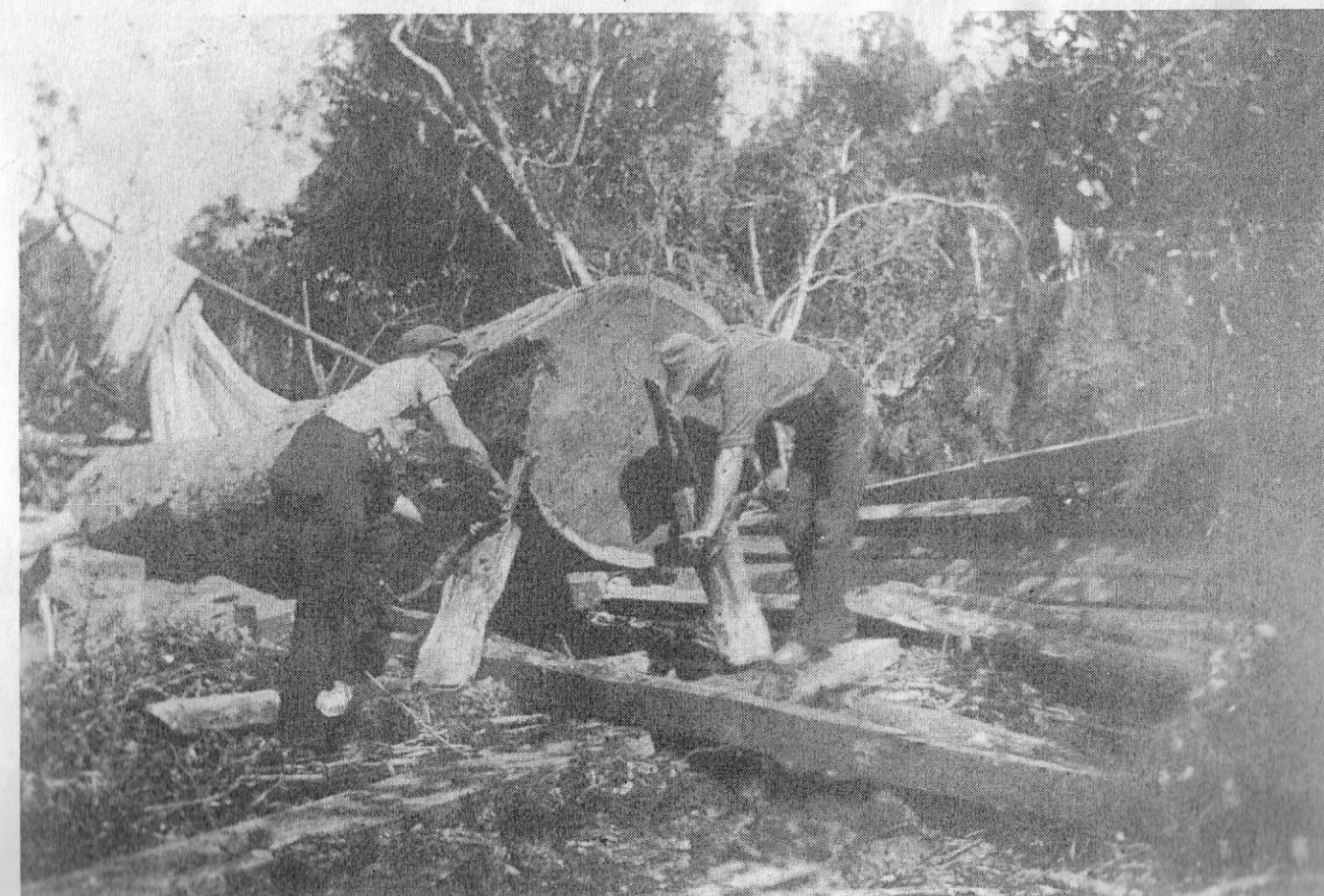
Felling with crosscut saw and moving log with timberjacks.
