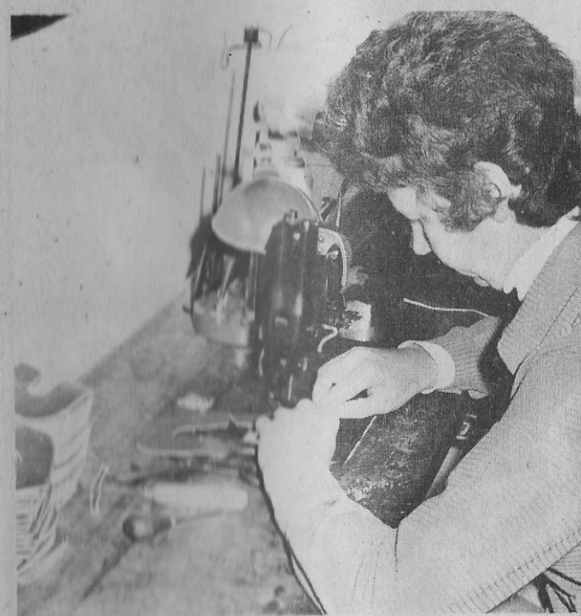
The uppers are sewn together on this machine.
