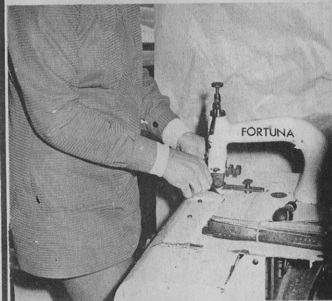
This operation is called Skiving. The outer edge of the straps are stitched to increase strength and to help stop stretching.
